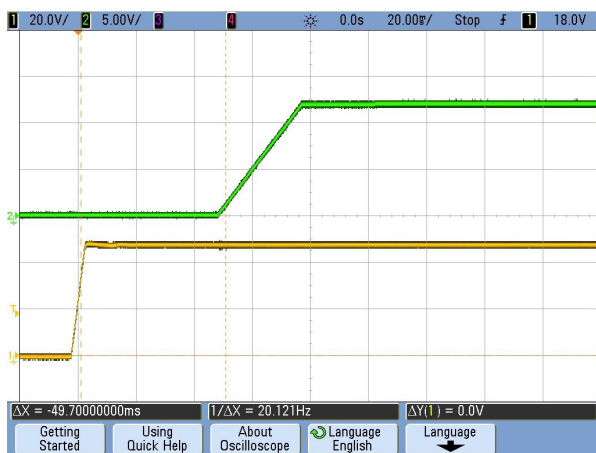
Figure 11. Vin Start-up Delay (CH2: Vout, CH1: Vin)
