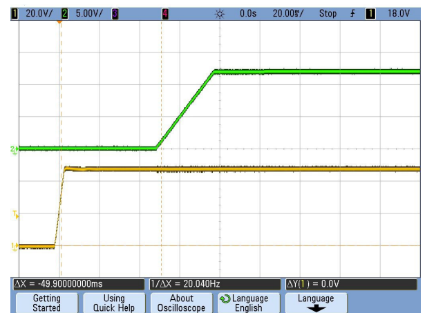
Figure 12. Vin Start-up Delay (CH2: Vout, CH1: Vin)
