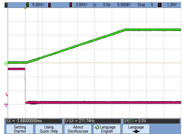
Figure 12. Vin Start-up Delay (CH2: Vout, CH1: Vin)
