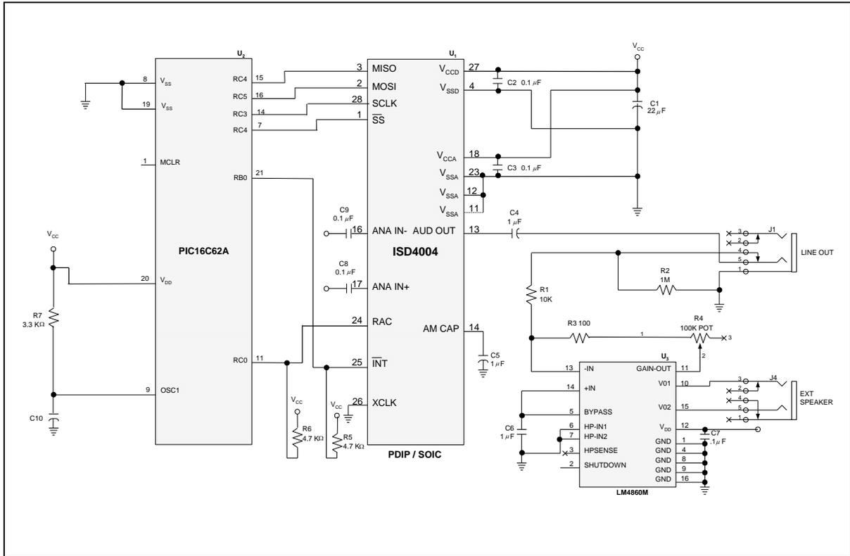
**FIGURE 11: APPLICATION EXAMPLE USING SPI PORT ON MICROCONTROLLER**
