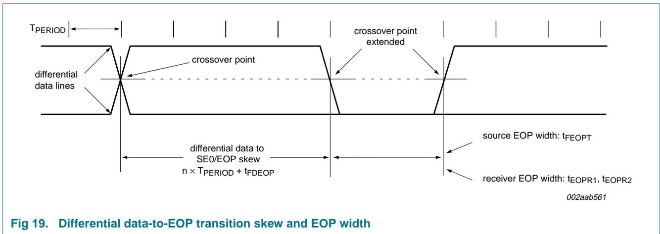
Fig 19. Differential data-to-EOP transition skew and EOP width
