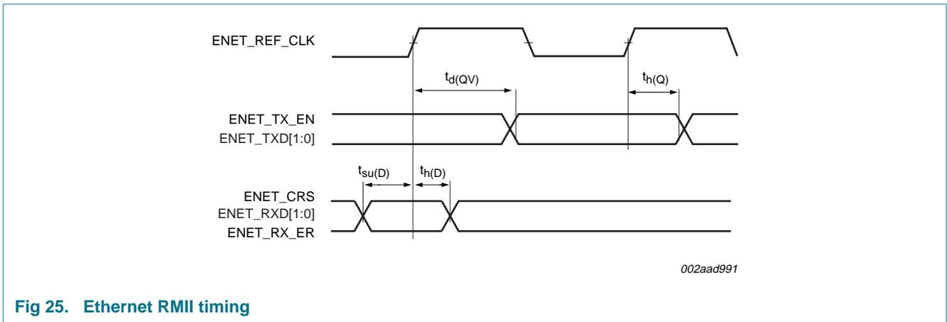
Fig 25. Ethernet RMI timing
