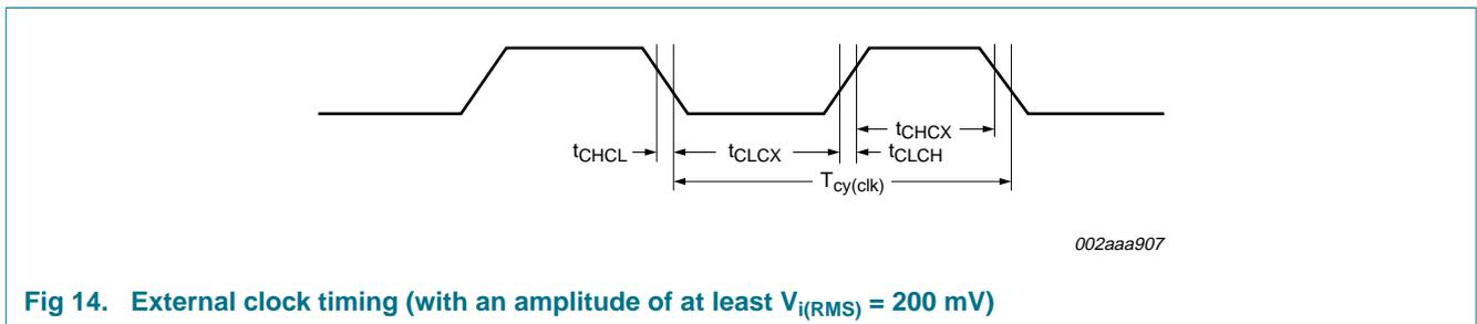
**Fig 14. External clock timing (with an amplitude of at least  $V_{i(RMS)} = 200\text{ mV}$ )**
