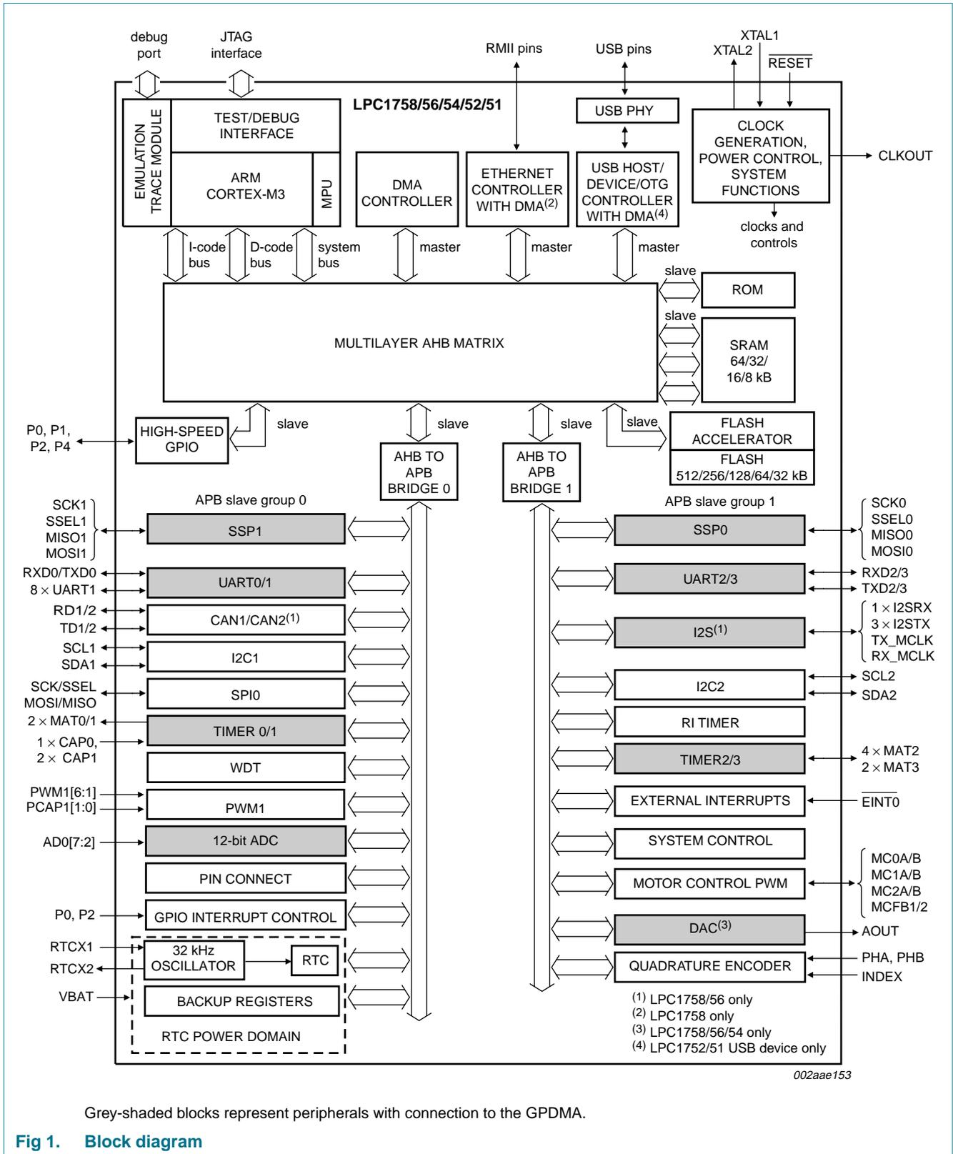
Grey-shaded blocks represent peripherals with connection to the GPDMA.
