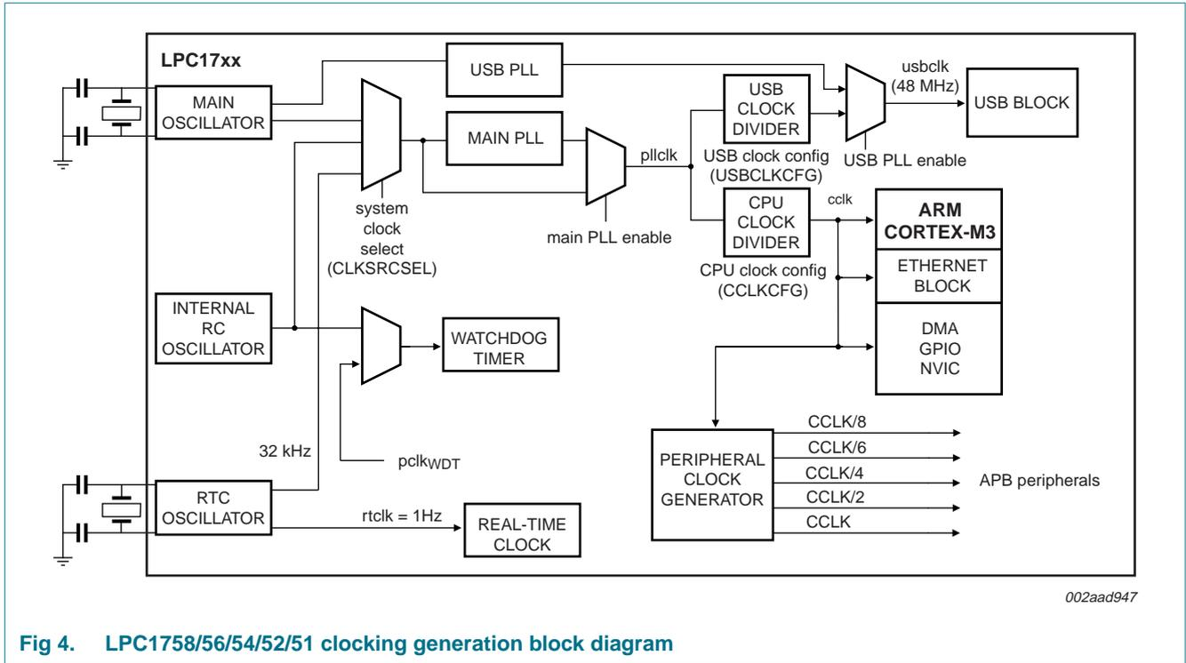
Fig 4. LPC1758/56/54/52/51 clocking generation block diagram
