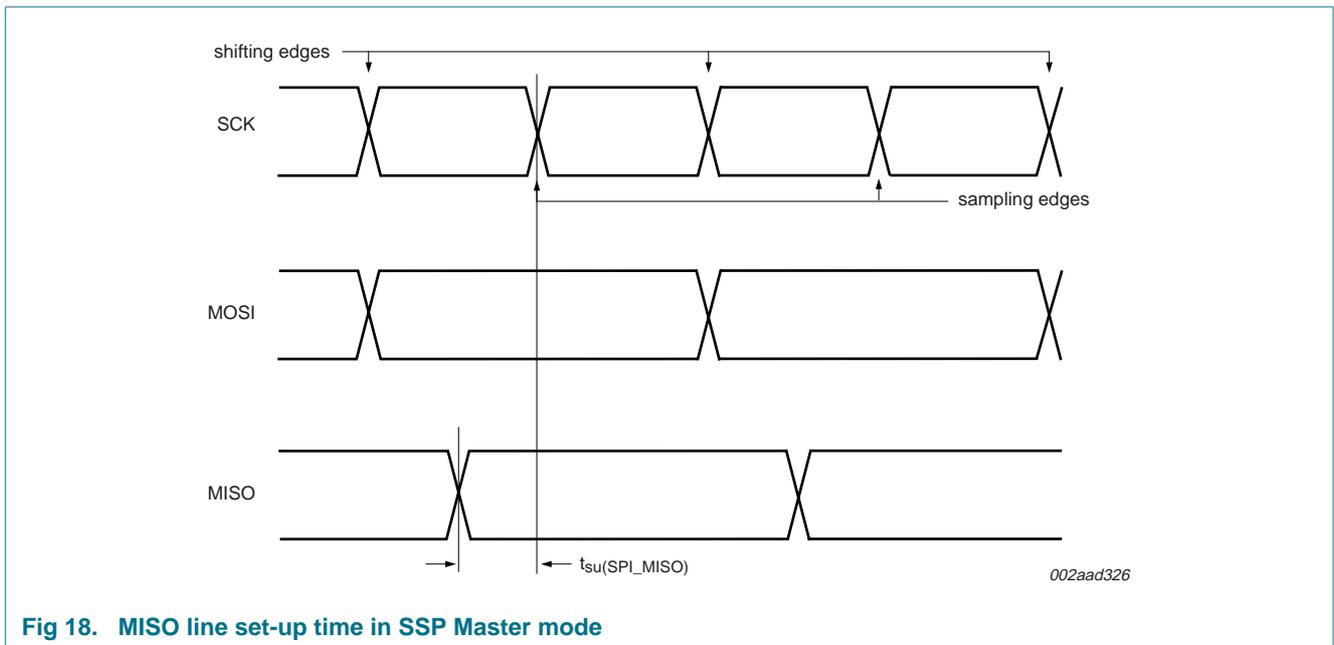
Fig 18. MISO line set-up time in SSP Master mode
