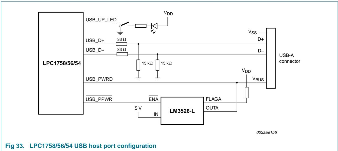
Fig 33. LPC1758/56/54 USB host port configuration
