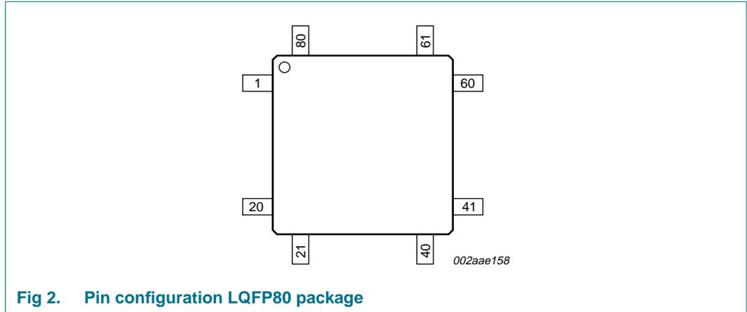
Fig 2. Pin configuration LQFP80 package
