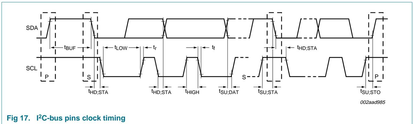
Fig 17. I<sup>2</sup>C-bus pins clock timing
