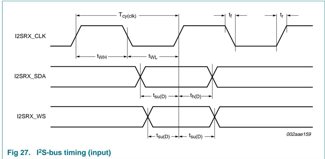
Fig 27. I<sup>2</sup>S-bus timing (input)
