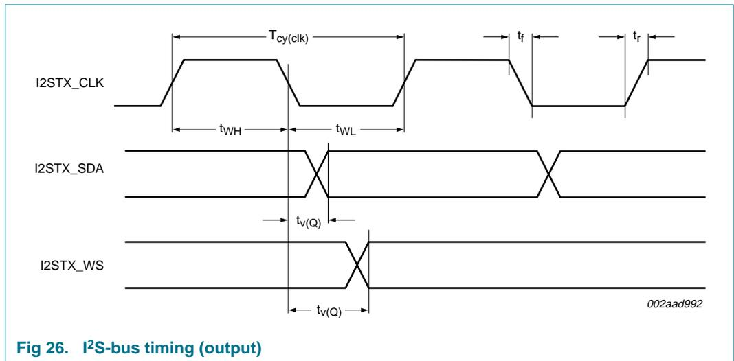
Fig 26. I<sup>2</sup>S-bus timing (output)
