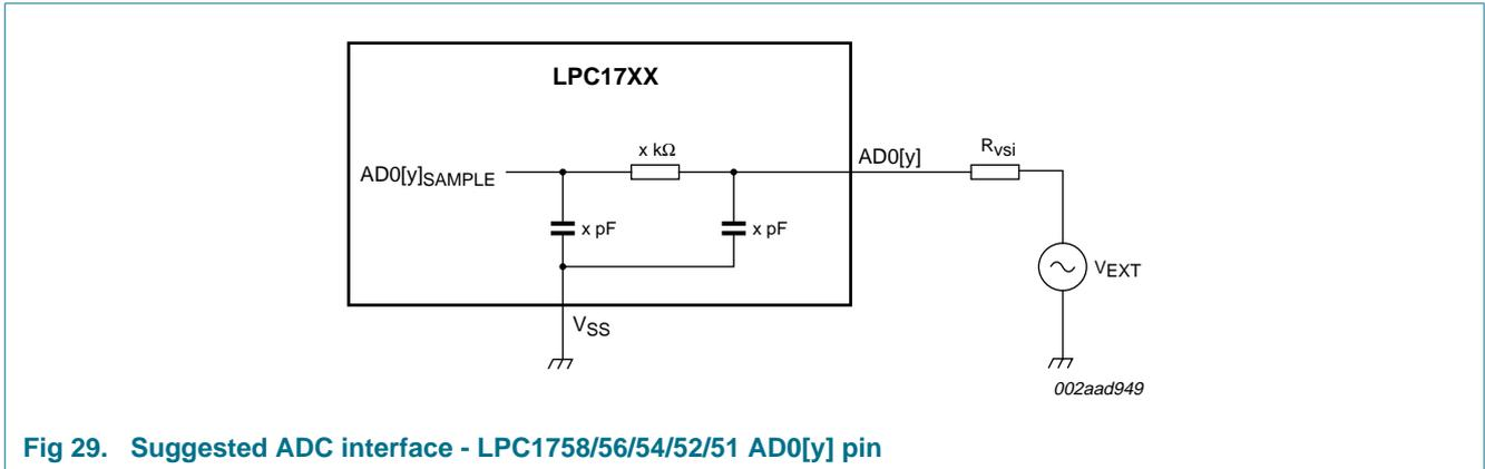
Fig 29. Suggested ADC interface - LPC1758/56/54/52/51  $AD0[y]$  pin
