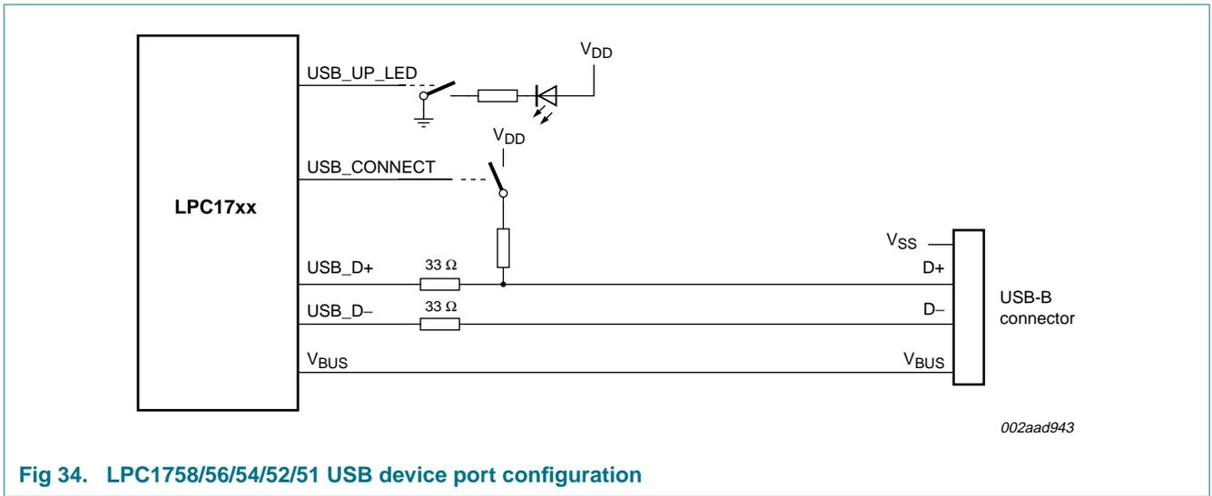
Fig 34. LPC1758/56/54/52/51 USB device port configuration
