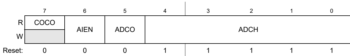
Figure 10-2. Status and Control Register (ADCSC1)
