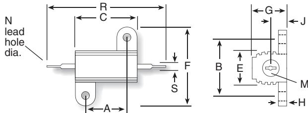
The 89 Series are high-performance axial-lead type resistors. These molded-construction metal-housed resistors are available in higher power ratings than standard axial-lead resistors and are better suited to withstanding vibration, shock and harsh environmental conditions.
