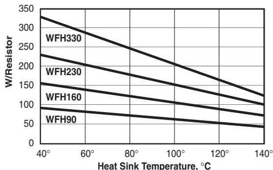
This graph shows the maximum wattage rating for each of the five possible resistors of standard size corresponding to the heat sink temperature. It is assumed that all resistors are equally loaded. Please consult us about non-standard lengths and resistor modules.
