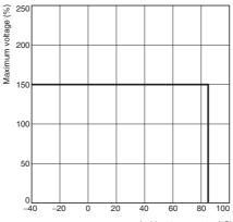
Ambient temperature (°C) "Maximum voltage" is the maximum voltage that can be applied to the Relay coil. Note:
