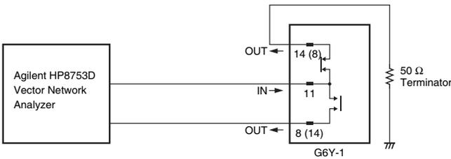
Terminals which were not being measured were terminated with 50 Ω.
