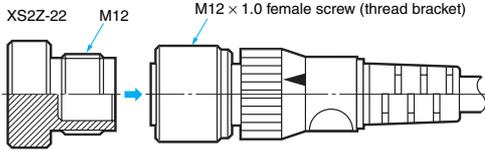
The Water-resistant Cover ensures IP67. When mounting the Water-resistant Cover to a Connector, be sure to apply a torque range between 0.39 and 0.49 N·m to tighten the Water-resistant Cover.
