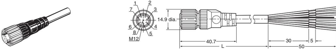
**XS2W Plug and Socket on Cable Ends (M12)**
