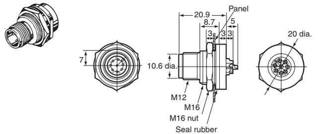
**XS2P-D822-2 Panel-mounting Socket (M12) with Solder Cup Pins and Front Lock**
