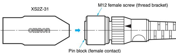
The Sputter Protective Cover protects the connector from weld sputter. Make sure it covers the entire connector.
