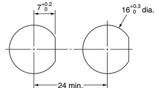
Note: The panel thickness is 1 to 4 mm.
