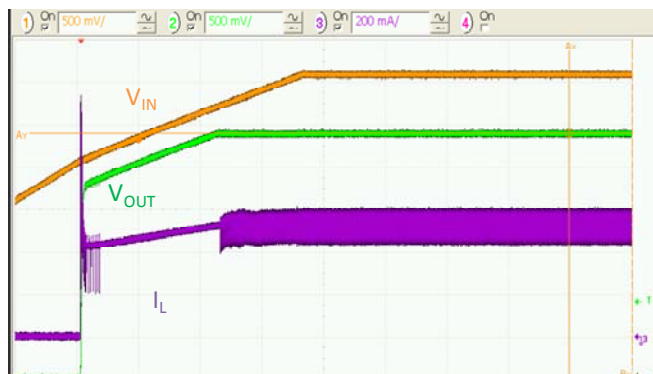
Figure 17. Startup Ramping V_{IN}=V_{EN} with 500mA Load, 1ms/div.
