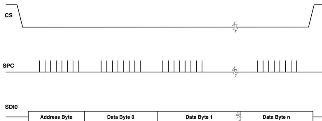
Figure 18. SPI 3-Wire Multi-Byte Read and Write Transactions
