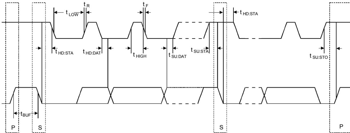
Figure 1 I<sup>2</sup>C Timing
