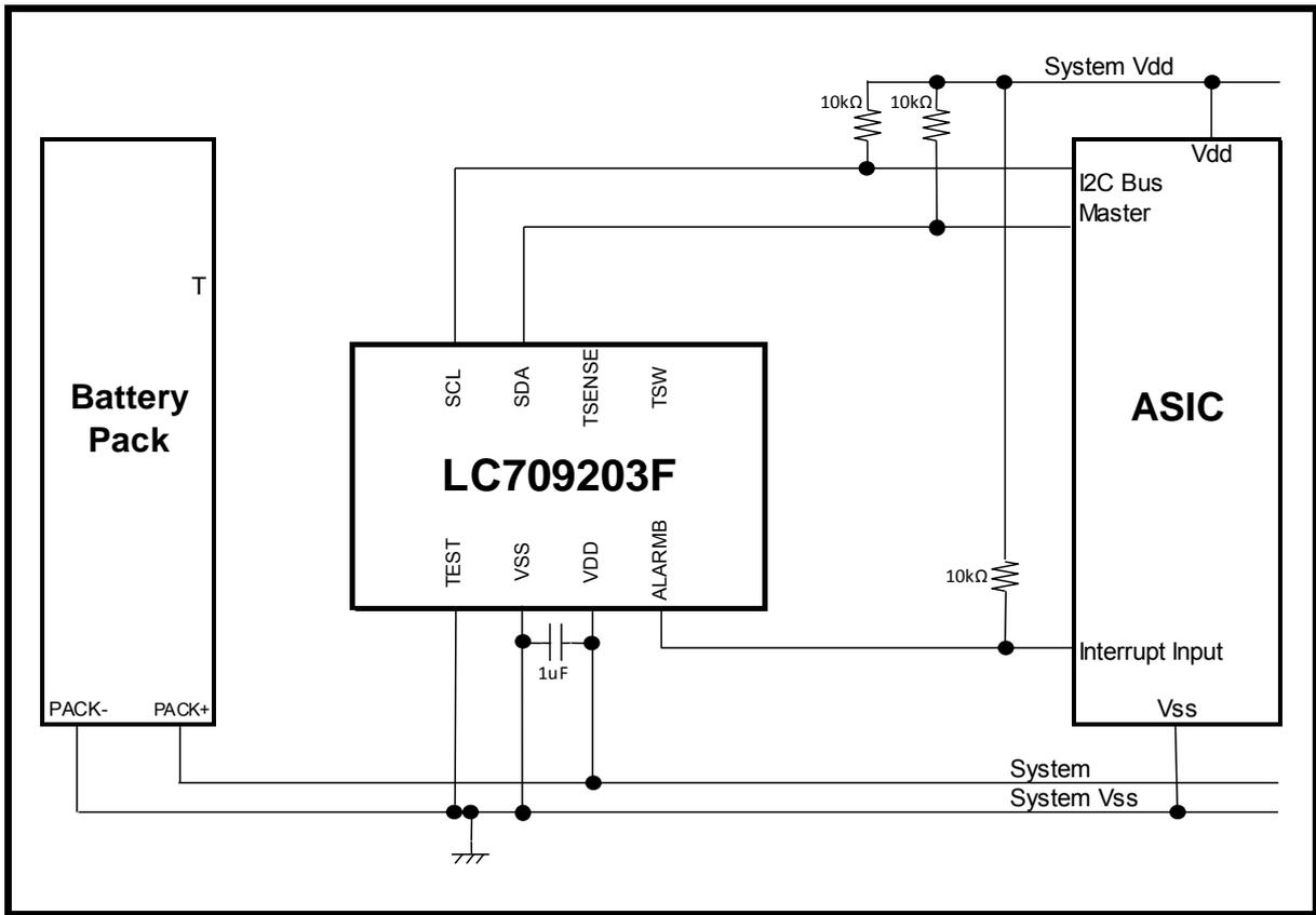
Figure 5 Example of an application schematic using LC709203F
