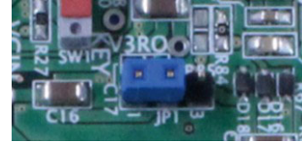
Figure 10. Jumper Switch JP1
