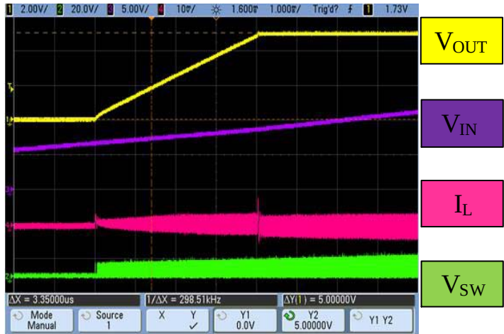
Figure 21. Start-Up Transition at No Load
