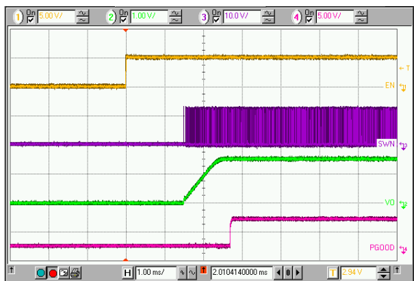
Top to Bottom: EN, SWN, V_o , PGOOD Figure 9. Powerup Sequence
