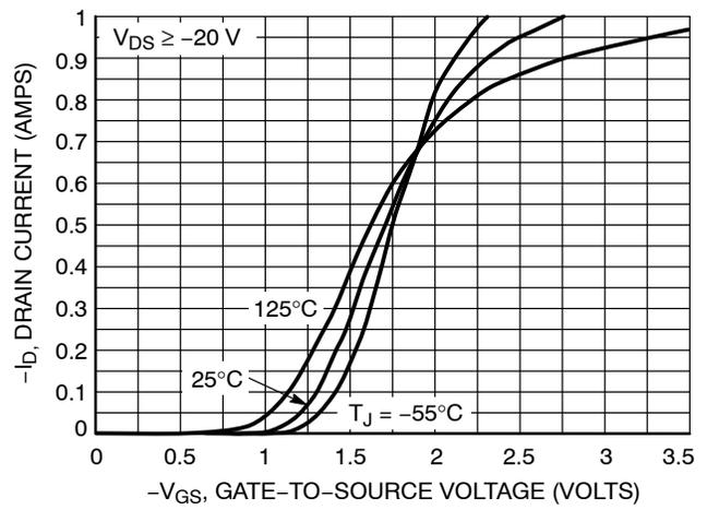
**Figure 2. Transfer Characteristics**
