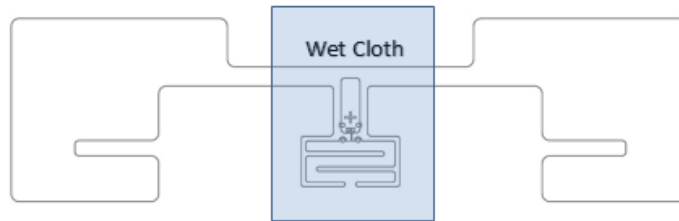
Figure 1. Moisture Contact Test Area
