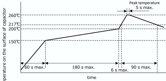
The model of MSL "2a" is changed into MSL "3" with this reflow condition.
