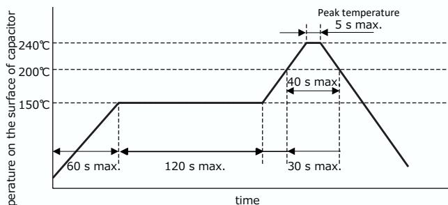
The cycles of reflow soldering : Twice
