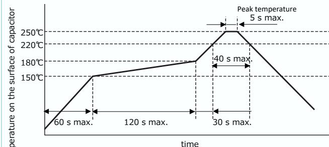
The cycles of reflow soldering : Twice
