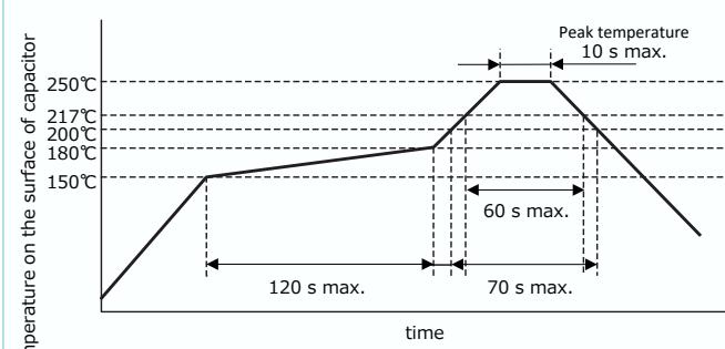
The cycles of reflow soldering : Twice
