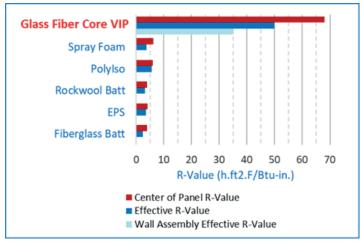
Center of panel R-Values determined using ASTM C1667. The Effective R-Value based on Panasonic calculations. Wall Assembly Effective R-Value determined by ASTM C1363, which takes into account edge effects in a specific Wall Assembly.
