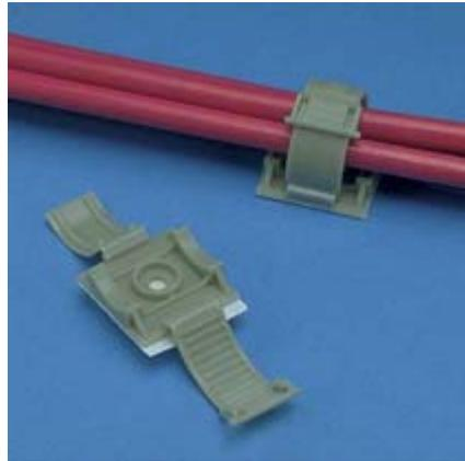
This clamp provides a fast and convenient method of securing bundles from .19" (4.8mm) up to .69" (17.5mm) diameter. It is available with adhesive backing or screw applied with one #6 (M3) screw.
