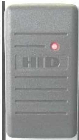
Figure 2-15 Bi-color LED in a Security Device
