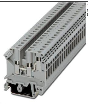
1-level terminal block with double connection on one side, cross section: 0.2 - 4 mm<sup>2</sup>, AWG: 30 - 10, width: 6.2 mm, color: gray
