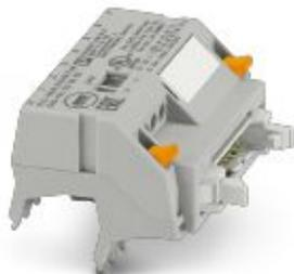
V8 adapter for 8 x PLC-INTERFACE (6.2 mm), controller: PLC system cabling of output cards, connection 1: Screw connection 1x, connection 2: IDC/FLK pin strip 1x 14-position, connection 3: Plug connection (Can be snapped onto 8x PLC-INTERFACE terminals), number of channels: 8, control logic: negative switching
