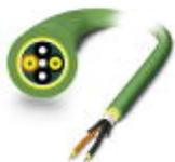
PROFINET HCS GI installation cable for assembly (IP20 heads only), suitable for drag chains, for indoor installation, gradient index fibers. Individual elements made from highly flexible FRNC material. Halogen-free, ozone and UV resistant with a polyurethane (PUR) outer sheath.
