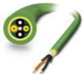
PROFINET HCS GI fiber cables, duplex 200/230  $\mu\text{m}$ , increased bandwidth for Ethernet applications in particular. Robust PUR outer sheath. Heavy version suitable for drag chains and indoor installation, sold by the meter without plugs
