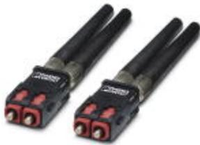
SC-RJ connector set for standard PROFINET PCF fiber cables with 2.2 mm diameter of the individual elements. Consisting of 2 duplex quick mounting connectors with bend protection for self-assembly.
