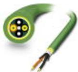
HCS-GI installation cable for assembly for fixed installation in the inner area, with gradient index fibers for the highest performance requirements, as well as individual elements made of highly flexible FRNC material. The cable is halogen-free, ozone and UV resistant and has a rugged polyurethane (PUR) outer sheath.
