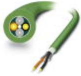
HCS PROFINET installation cables that can be assembled for fixed installation indoors and outdoors (direct underground installation not permitted) with individual elements made from extremely hard-wearing polyamide (PA). The cable is halogen-free, ozone and UV resistant and has a PVC outer sheath.
