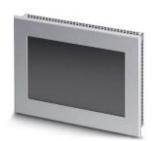
Touch panel with 17.8 cm/7" TFT-display (analog resistive (polyester)), 800 x 480 pixel(s) (WVGA), 262144 colors, Arm<sup>®</sup> Cortex<sup>®</sup>-A8, 800 MHz, 2x USB host 2.0, 1 x Ethernet (10/100 Mbps), RJ45, Windows<sup>®</sup> Embedded Compact 7 and user software: Visu+ / AX OPC Server. (bus system: without)
