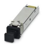
The small form-factor plug-in module is a plug-in fiber optic interface with a data transmission speed of 1000 Mbps, which is used in Gigabit Ethernet. Fiberglass module with a wavelength of 850 nm.
