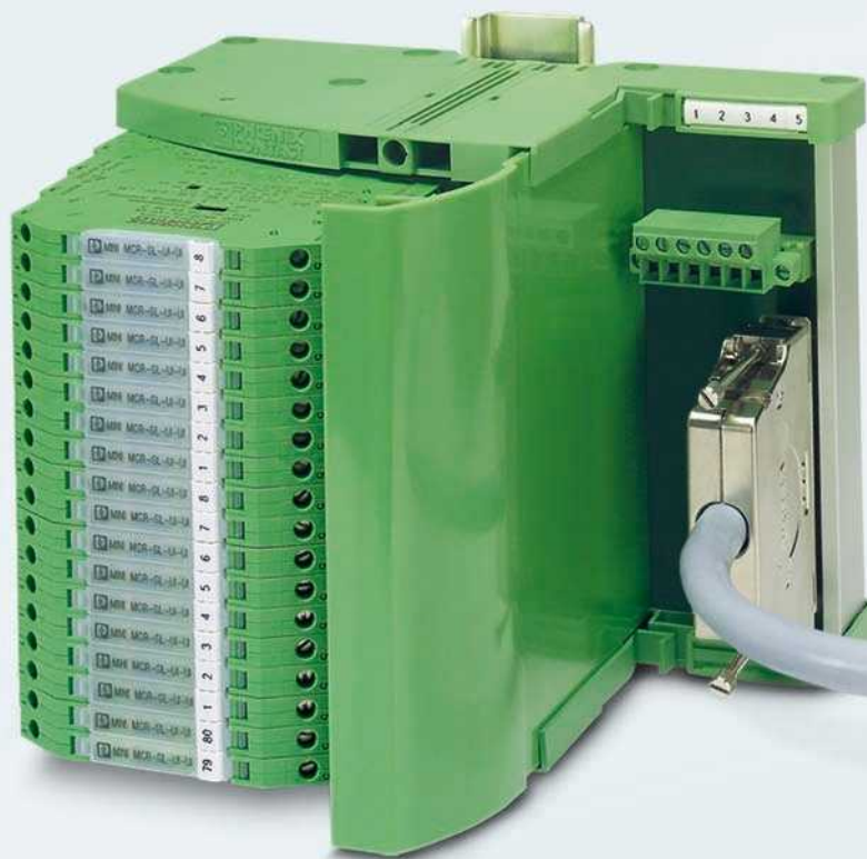
Hot-swappable system cabling with the termination carrier
