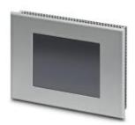
Touch panel with 14.5 cm (5.7") graphics-capable C-STN display, 125 colors,  $320 \times 240$  pixels, 1 x Ethernet, 2 x USB, and integrated runtime of the Visu+ visualization software.
