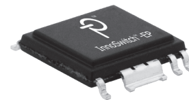
Figure 2. High Creepage, Safety-Compliant eSOP Package.
