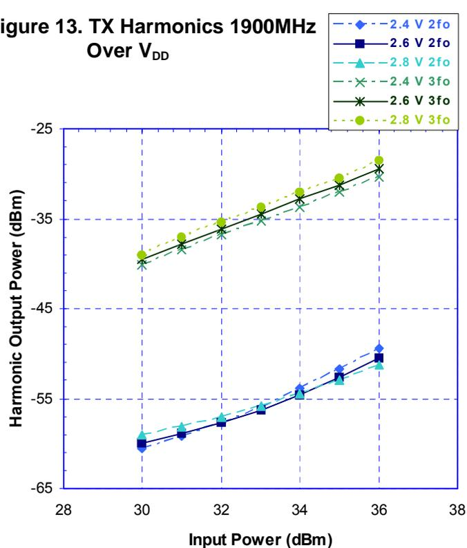
Typical Performance Data @  $V_{DD} = 2.6\text{ V}$ ,  $25\text{ }^\circ\text{C}$  (Unless otherwise noted)
