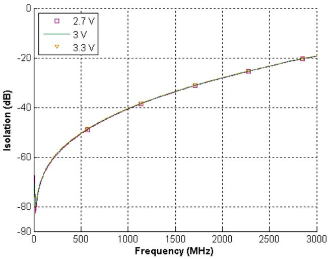
Figure 8. Isolation: RF1 - RF2 @ 3.0V
