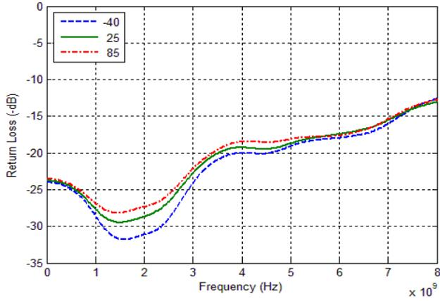
**Figure 9. RFC Port Return Loss vs.  $V_{DD}$**
