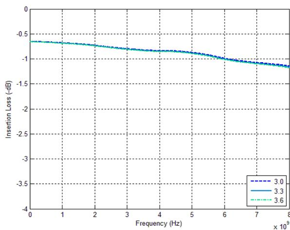
Typical Performance Data @ 25°C and  $V_{DD} = 3.3V$ , unless otherwise specified
