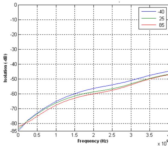
**Figure 11. Isolation: RFX-RFX @ 25 °C**
