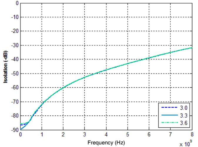
**Figure 11. Isolation: RFX-RFX vs Temp**
