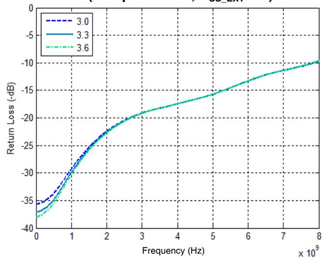
**Figure 17. Terminated Port Return Loss vs Temp**
