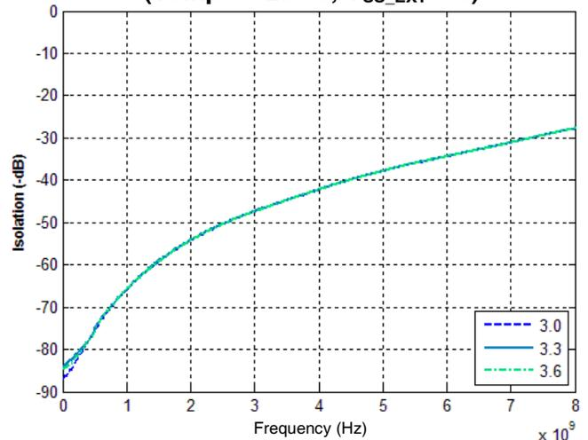
**Figure 13. Isolation: RFX–RFC vs Temp**
