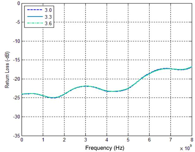
**Figure 15. Active Port Return Loss vs Temp**
