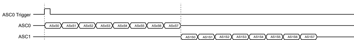
Figure 17-5. ASCx, ADCCTL.ADCMODE = 011b, 110b
