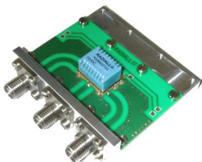
Relay soldered on Test Fixture (2)
