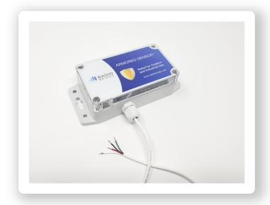
The 4-20mA sensor uses a 10-bit ADC to measure an analog value between 4-20mA and provides 10uA of resolution.
