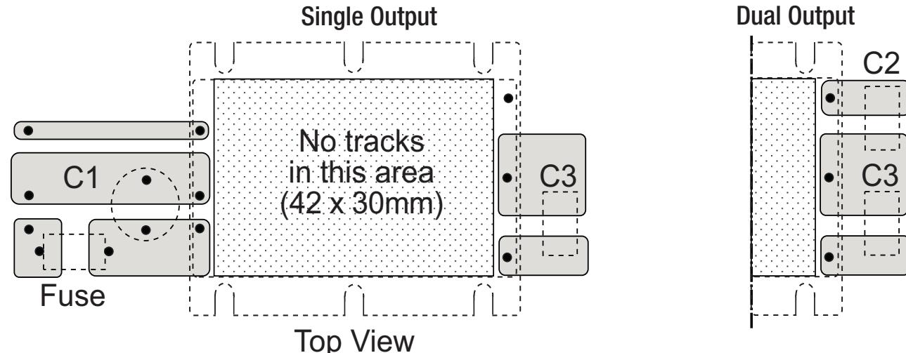
Input Fuse is recommended, but optional. Recommended fuse rating = double maximum input current, time delay type.
