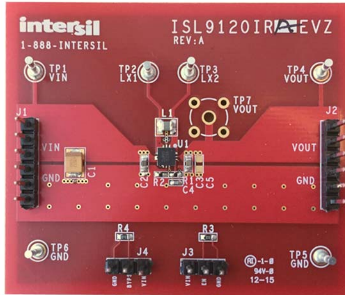
FIGURE 4. ISL9120IRA-EVZ EVALUATION BOARD
