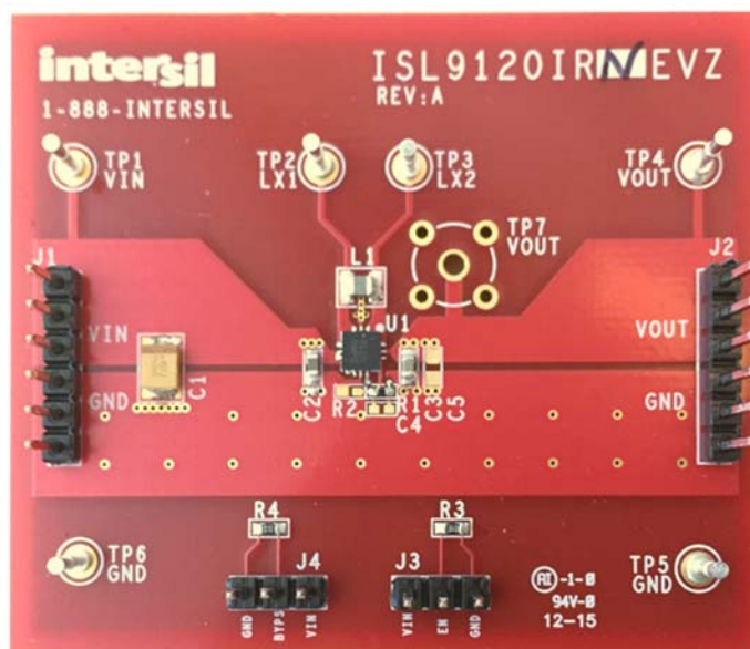
FIGURE 6. ISL9120IRN-EVZ EVALUATION BOARD
