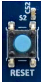
Figure 16 Reset Switch (S2) on Target Board
