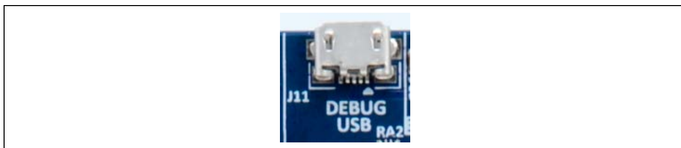
Figure 4 USB Debug Connector (J11), TP3, and TP4 on the Target Board
