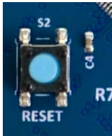
Figure 18. Reset Switch (S2) on Target Board
