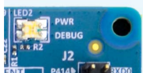
Figure 10. LED2 on Target Board (Top)
