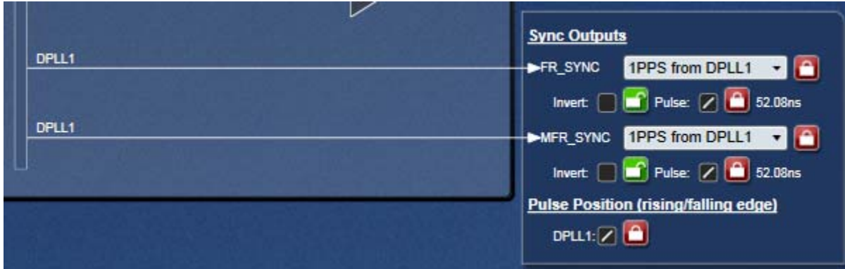
Figure 17. Configure MRSYNC and MRFSYNC
