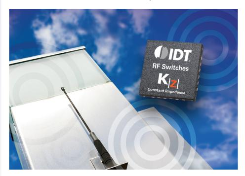
$K_{|Z|}$ , Constant Impedance: IDT's  $K_{|Z|}$  innovation improves system hot switching ruggedness, minimizes LO pulling in VCOs, and reduces phase and amplitude variations in distribution networks. It is also ideal for dynamic switching between multiple amplifiers while avoiding damage to sensitive upstream / downstream devices such as PAs and ADCs.
