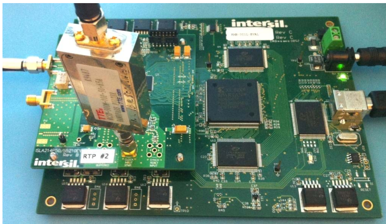
FIGURE 3. ISLA214P50-55210EV1Z DAUGHTERBOARD ON KMB-001 MOTHERBOARD
