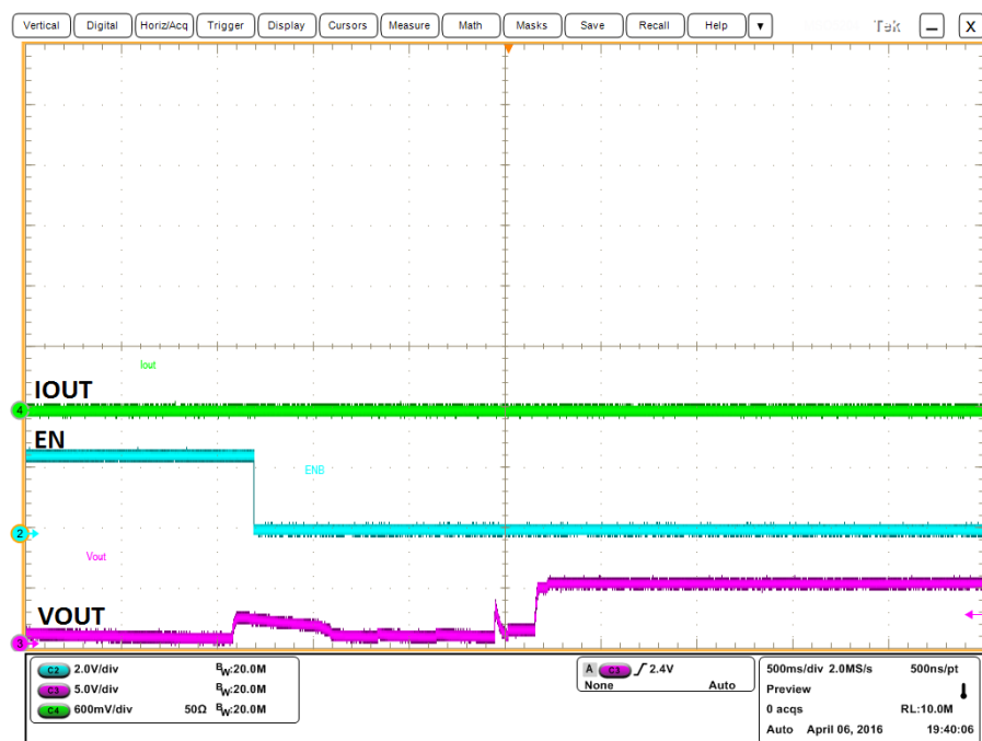
Figure 13. No Load Start-up by Rx Enable Signal (Ch2=EN, Ch3=Vout, Ch4=Iout)
