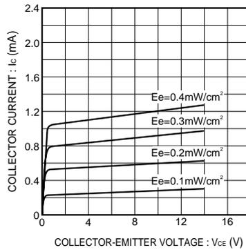
Fig.2 Output characteristics
