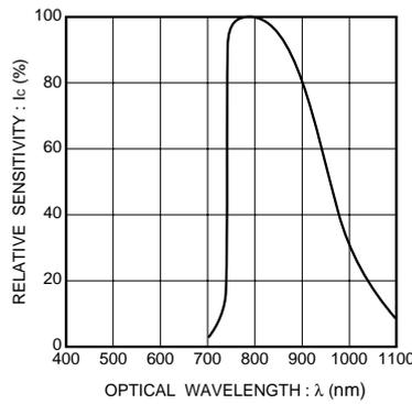
Fig.5 Spectral sensitivity
