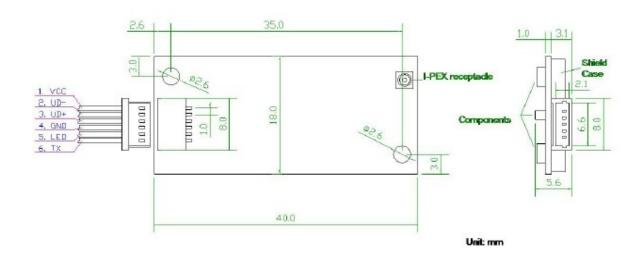
6-pin 2.0 mm pitch male header -Top View
