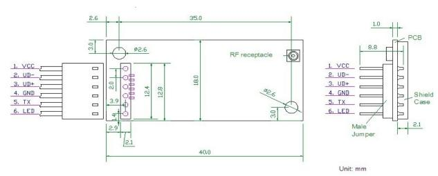
For custom applications: the direction of the male header can be mounted upside down, please contact Sagrad Inc. for availability.
