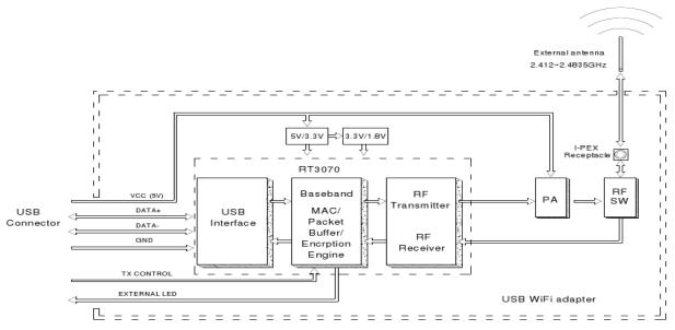
System Block Diagram of SG901-1059B-3.3 WLAN Module
