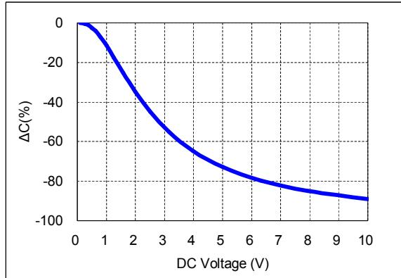
4) Bias TCC characteristics (Agilent 4284A, 1kHz, 1.0Vrms, 5Vdc)
