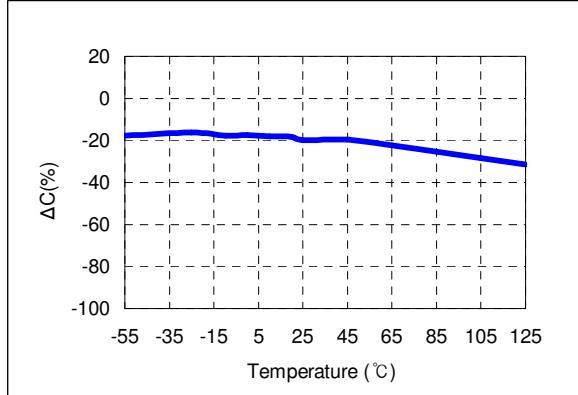
5) AC voltage characteristics (Agilent 4284A, 1kHz)
